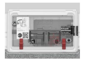
**Proven reliability:** the TECE Uni cistern comes pre-assembled and sealed ex works. It only needs to be connected to the pipes during the shell installation phase. You only have to open it during fine installation – and construction debris remains safely out of the box.
